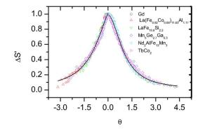
FIG. 1. (Color online)  $\theta$  dependence of  $\Delta S'$  for the studied samples for typical field changes (0–1, 2, 3, 4, and 5 T); the solid line is the fit to Eq. (2).
