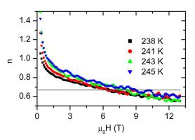
FIG. 3. (Color online) Field change dependence of *n* in the vicinity of  $T_C$  for LaFe<sub>10.8</sub>Si<sub>2.2</sub> compound; the solid line is the n=2/3 reference.
