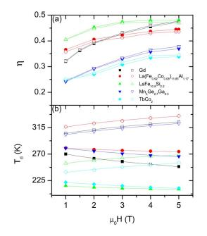
FIG. 4. (Color online) Field change dependence of (a)  $\eta$  [the closed symbols are for experimental data and the open symbols for the results of Eq. (2); the lines are a guide for the eye] and (b)  $T_{ri}$  (*i*=1,2) (the closed symbols are for  $T_{r1}$  and the open symbols are for  $T_{r2}$ ; the lines are a fit to a power law of the field).
